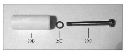
9. Check plunger surface (29B). If plunger pipe is worn out, loosen tension screws (29C) and pull off plunger pipe to the front. Clean front surface of plunger (25) thoroughly. Apply a thin coat of Loctite to the tension screw threads (29C). Note: Care must be taken that no glue gets between the plunger pipe (29B) and the centering sleeve (29A). Add new copper ring (29D).
